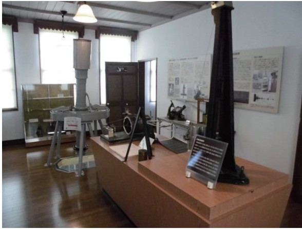
Fig. 7 The FZT (Floating Zenith Telescope) and Seismometer
