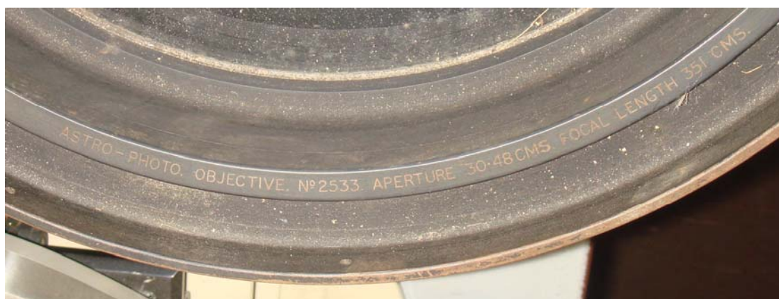
写真3 ASTRO-PHOTO. OBJECTIVE. No. 2533 APERTURE 30.48CMS. FOCAL LENGTH 351CMS. の刻印
