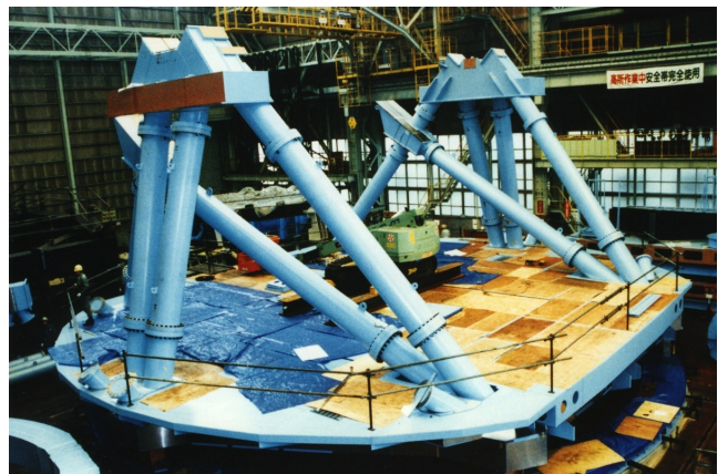
Telescope mount. Two tripods are ready to support the elevation axis of the telescope.
