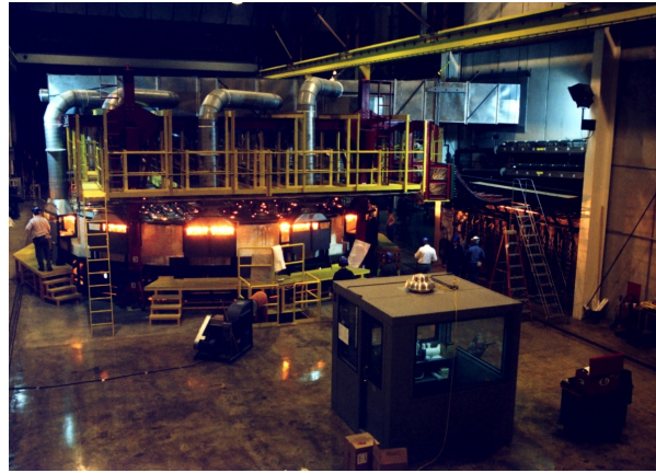
Then fused in a furnace to make 8 m mirror blank.
