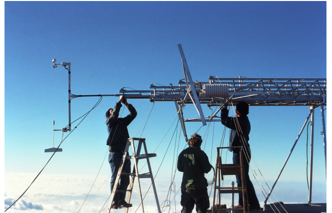
Sensors for measuring the atmospheric turbulence are set at several heights from the ground-level. Now, our engineers are setting the top-part sensor. ©NAOJ
