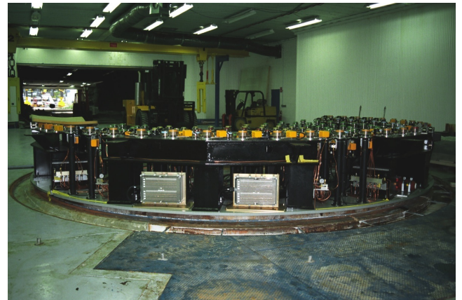
Support arms to be used during the fabrication of mirror.
