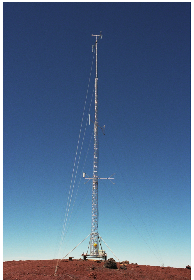
Thirty-meter tower to measure the height of the surface turbulence layer. ©NAOJ
