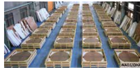
A special glass with an extremely low thermal expansion rate is used for TMT's primary mirror segments, which comprise part of Japan's contribution. As of March 2024, 356 mirror blanks have been produced.
